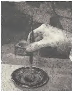
Below: Using a brush and abrasive grains to produce a satin or French gray finish on polished metal. The brush can be manipulated in various ways to produce different effects.
